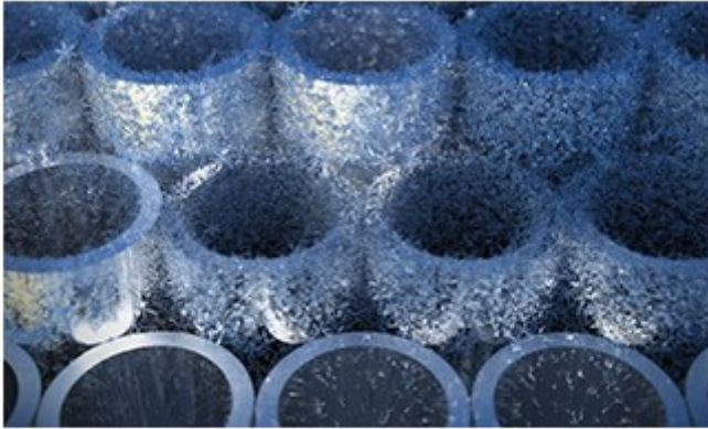
Metallic solid-state refrigerant tubes used for elastocaloric cooling, an environmentally friendly refrigeration technology. Credit: Jiaqi Dai/Maryland Engineering
