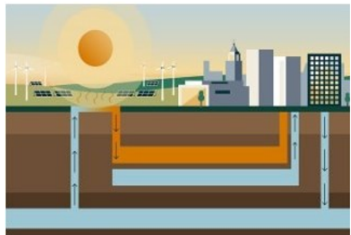
ATES uses naturally occurring underground water to store energy that can be used to heat and cool buildings. Credit: Jenny Nuss/Berkeley Lab
