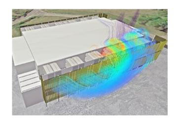
CFD simulations show airflow around the exterior of a data center. Credit: Future Facilities | Data Center Frontier
