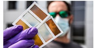
NREL's thermochromic window technology has advanced to have more tint colors. Credit: Dennis Schroeder, NREL
